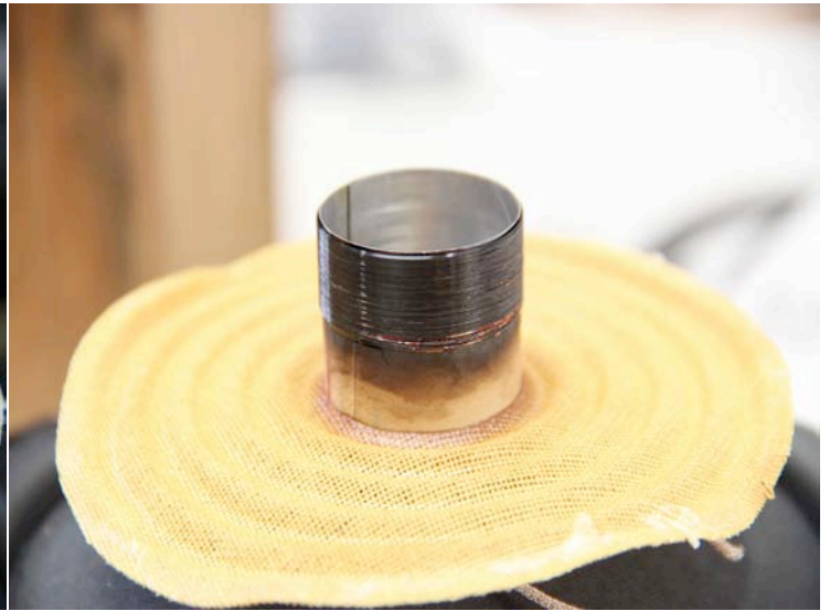
Damaged Speaker Voice Coil
