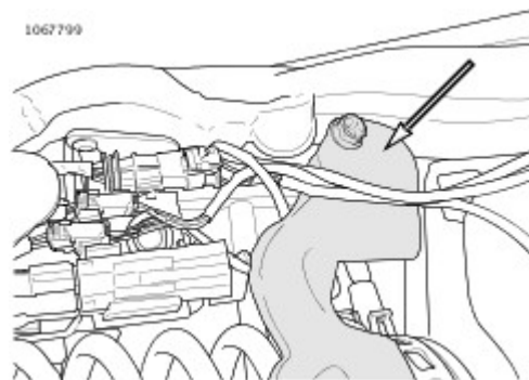
Figure 25. Siren Pager Antenna Wire Routing: (Rear tire and splash guard removed for clarity)
