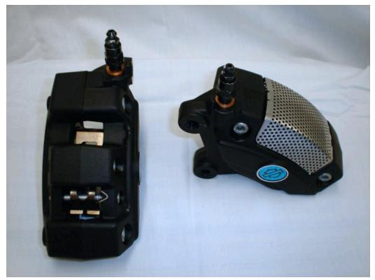
In these two views above we can also see the brake pad spring, pad pin, and pad pin retaining clip.
