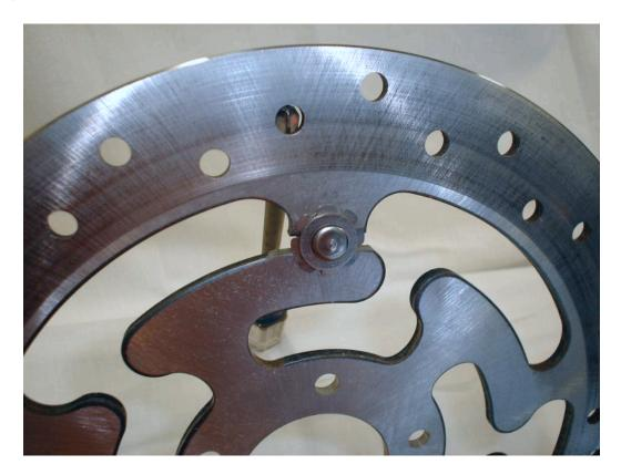
Installation of the rotors begins with mounting the appropriate (right or left) disc to the wheel hub with new T40 TORX bolts. If purchased from Dealer, these bolts already have thread locker applied. In recent years, the factory Service Manual would have us mount the rotors in the same location on both sides of the wheel. In fact, there was an entire section on **BRAKE DISC LOCATION AND ALIGNMENT**. From the '07 Service Manual:
