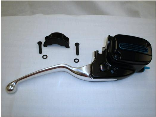
Note the blue rubber plug that's barely visible at the master cylinder outlet port. Since this was a take-off unit, the reservoir was still filled with brake fluid and the rubber plug had it sealed. This proved to be a big plus since it saved me the time of bench bleeding the unit. For anyone purchasing a new or un-filled master, I would highly recommend filling the unit on the bench and getting some fluid in the pump assembly so as to create
