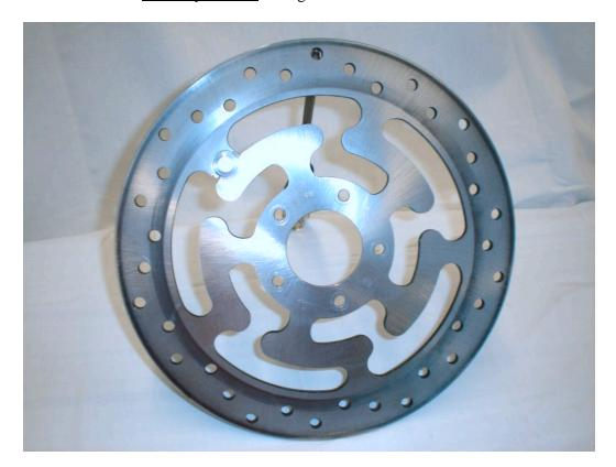
Also note the button at the 10-11 o'clock position. Some initially thought this was part of the ABS Braking System but "unofficial" sources call it a **whine-damping button**. Hear is a view of the back-side of the rotor and "button":
