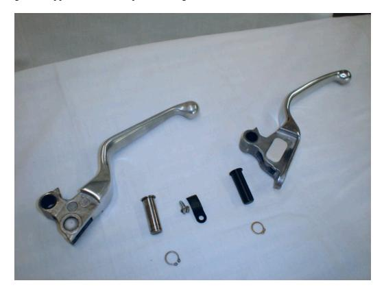
Next is the bottom side of clutch levers. As noted, anti-rattle spring and screw are common to both.
