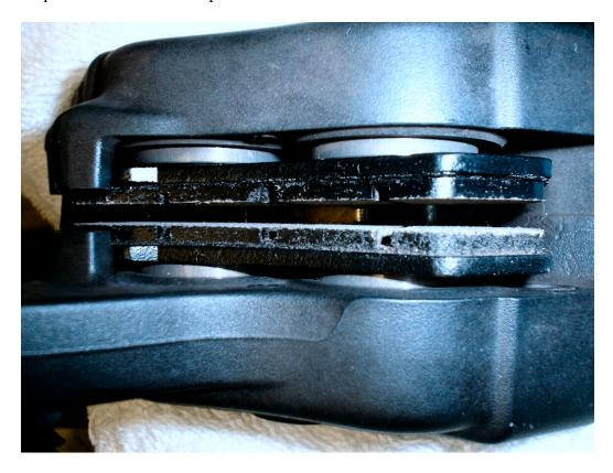
6. Turn caliper over and verify that pad pin tabs are centered under the forks of the pad spring.
